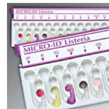
Micro-ID Listeria Identification System panel w/inoculated wells.
