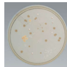
Settling Plate Tryptic Soy Agar w/growth.
