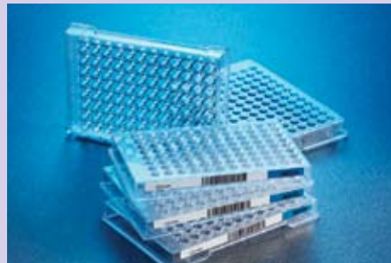
The Anaerobe MIC format offers laboratories an easy alternative to labor-intensive agar dilution procedures.
