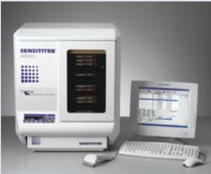
Affiliated Laboratory, Inc. used the automated Sensititre ARIS 2X System, along with Sensititre MIC plates, to evaluate oxacillin resistance in SA and CoNS.
